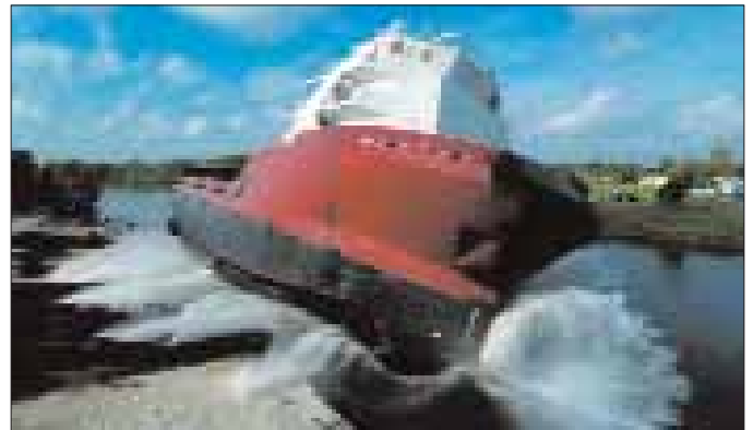
First of the Rigdon's GPA 654 PSVs being side-launched at Bollinger shipyard
